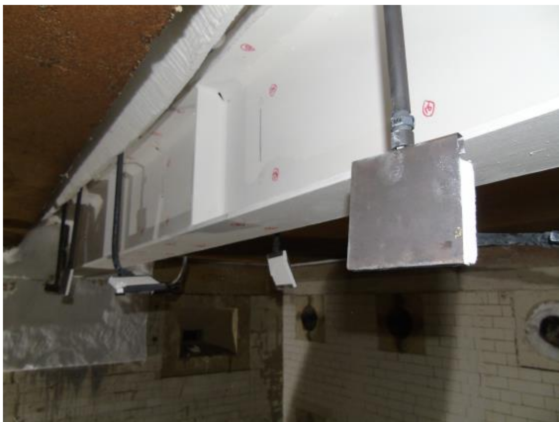
Photo D.4 Test 1: Loaded beam with minimum protection thickness before the test
