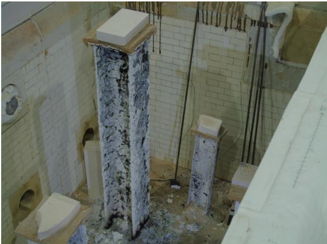
Photo D.18 Tall column after the test
