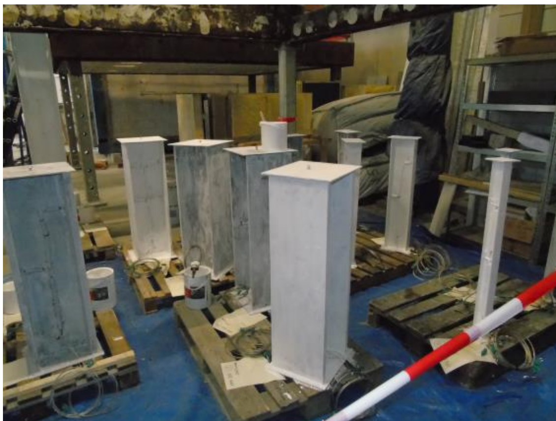
Photo D.3 Application of the coating on the short columns
