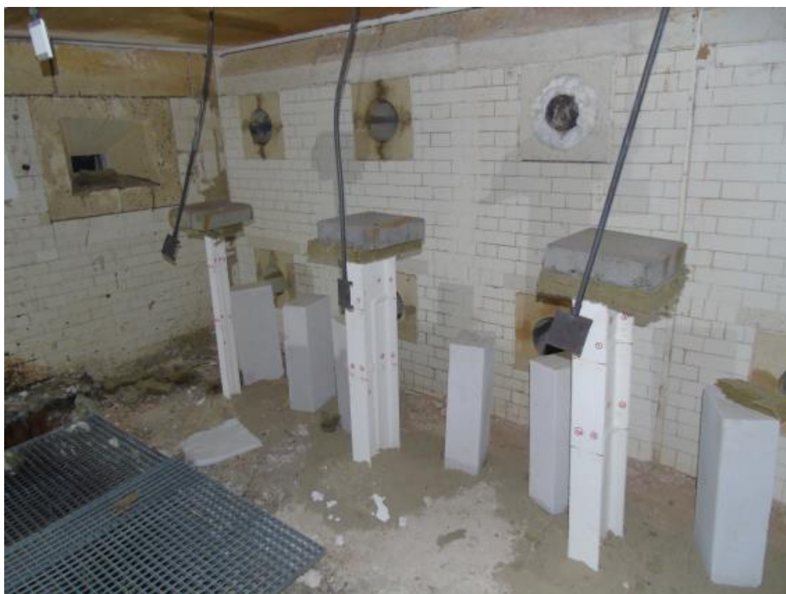
Photo D.10 Test 2: Some of the unloaded columns before the test
