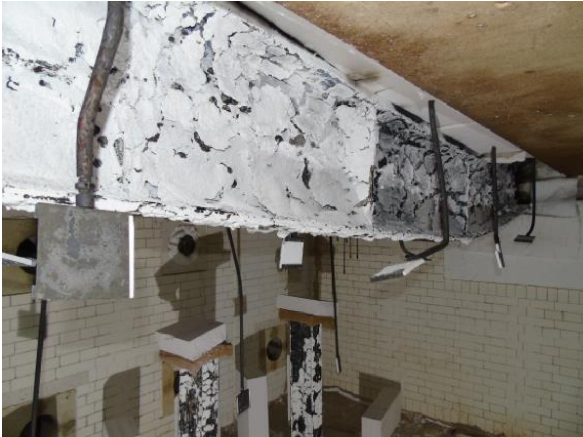
Photo D.11 Test 2: Loaded beam with maximum protection thickness after the test (1)
