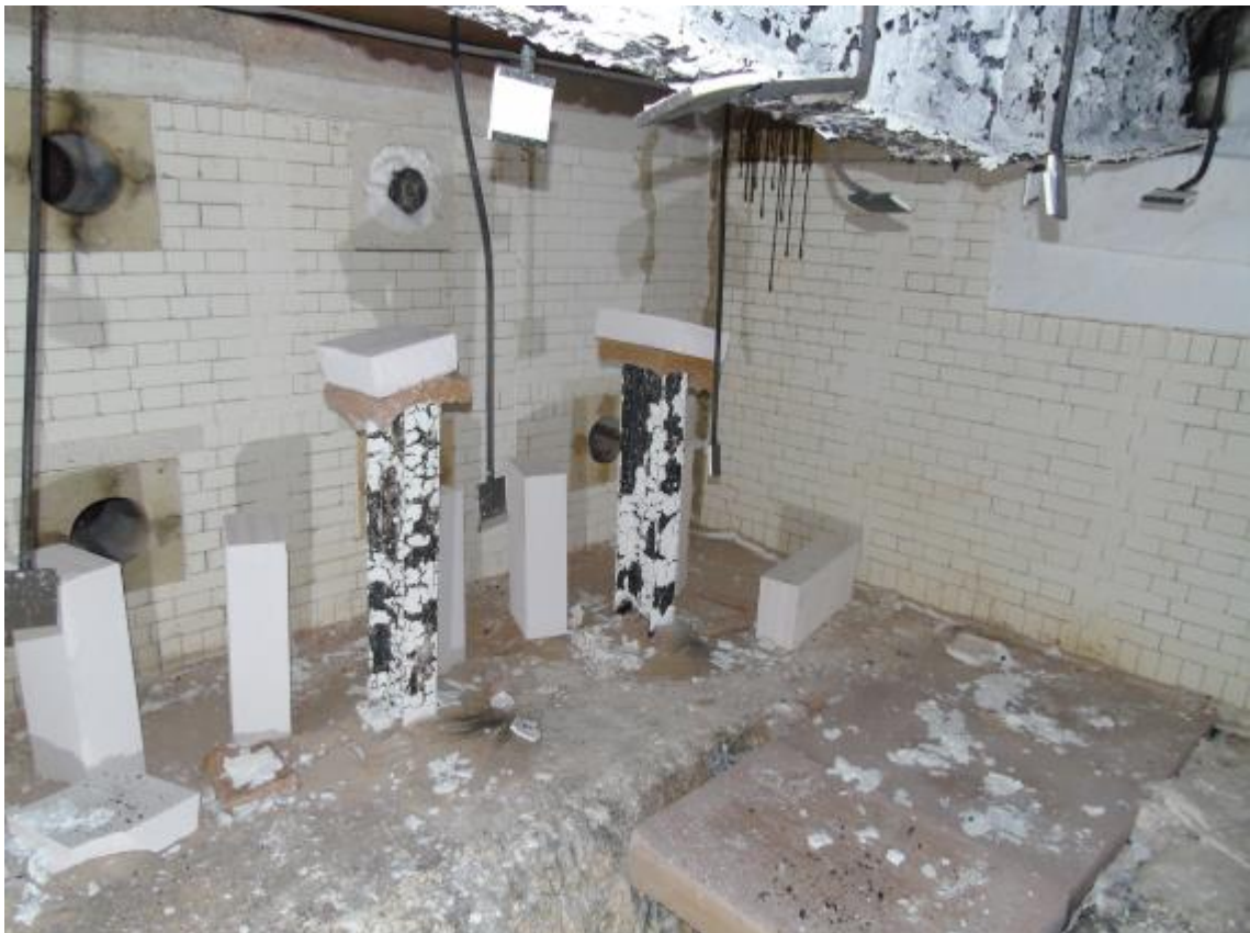
Photo D.14 Test 2: Some of the unloaded columns after the test
