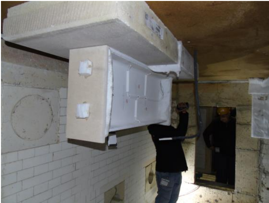
Photo D.5 Test 1: Reference beam with minimum protection thickness before the test
