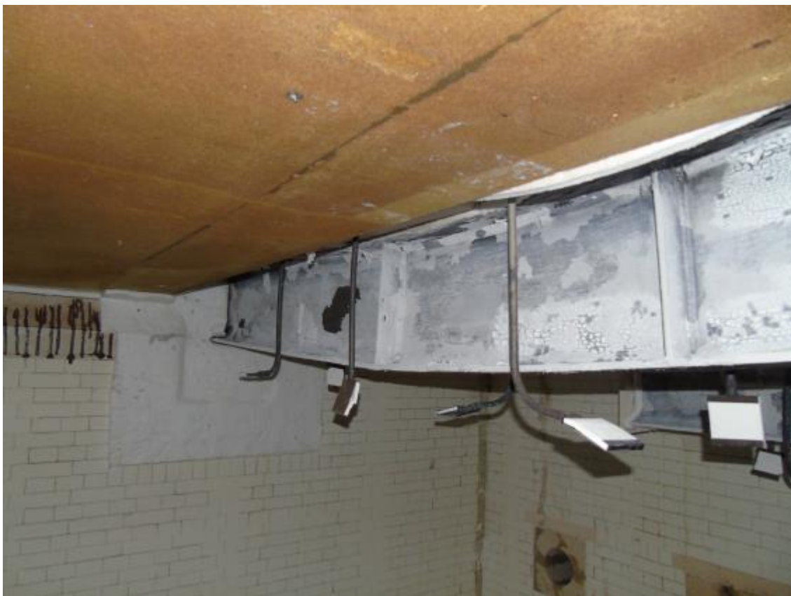
Photo D.6 Test 1: Loaded beam with minimum protection thickness after the test
