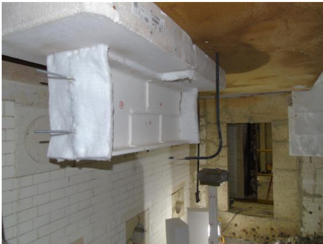
Photo D.9 Test 2: Reference beam with maximum protection thickness before the test
