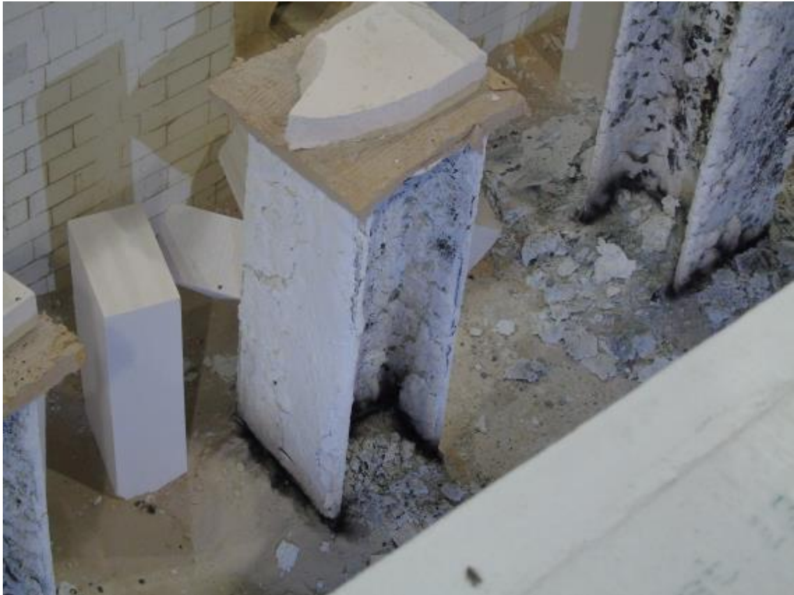
Photo D.17 Some of the unloaded columns after the test (2)
