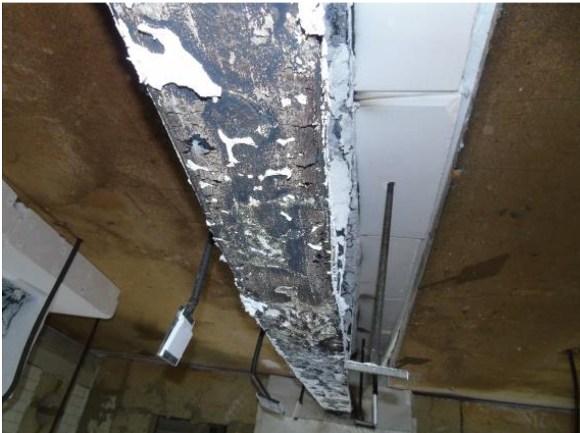
Photo D.12 Test 2: Loaded beam with maximum protection thickness after the test (2)
