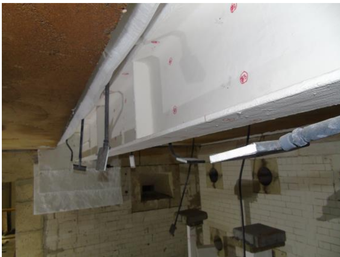
Photo D.8 Test 2: Loaded beam with maximum protection thickness before the test
