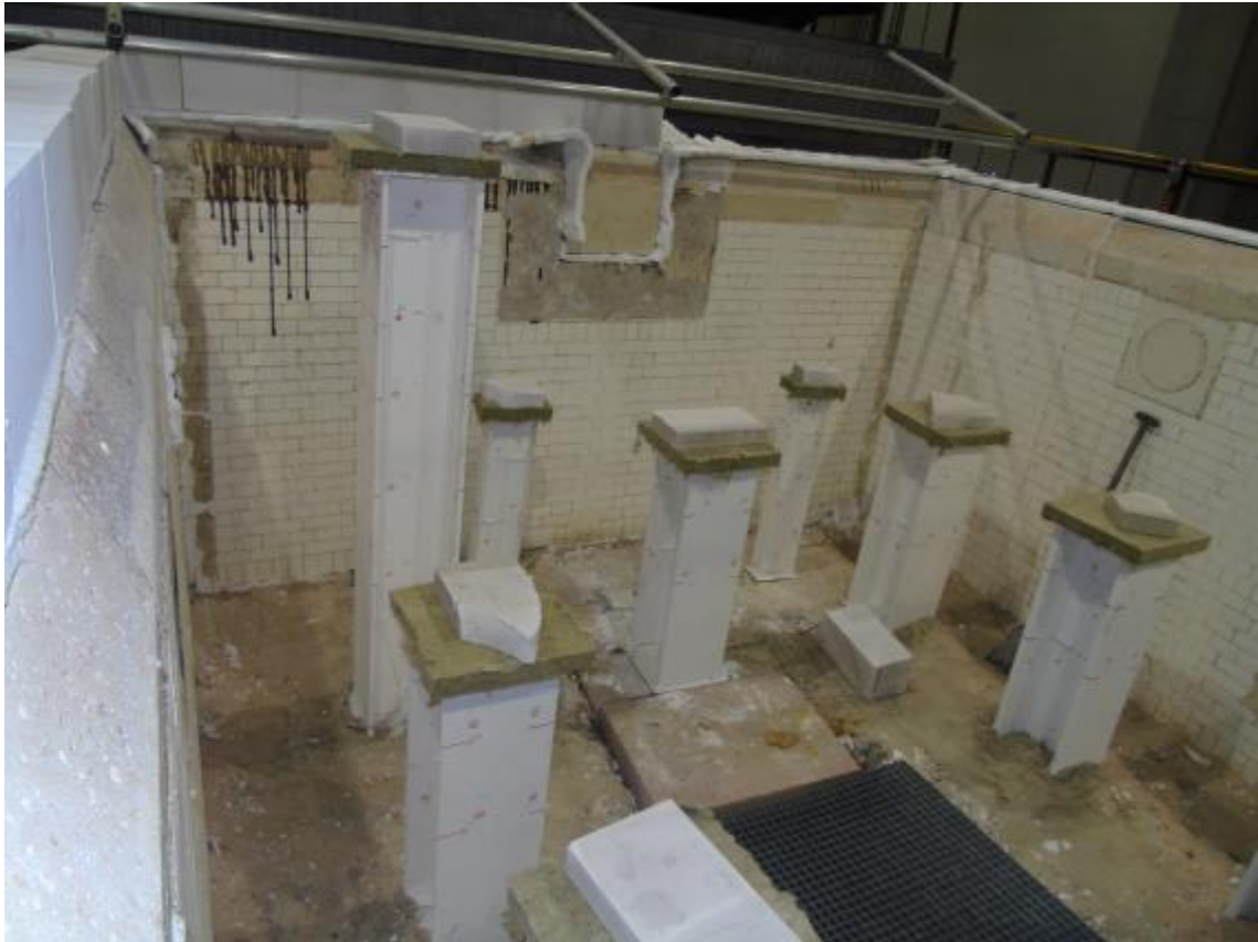
Photo D.15 Test 3: Unloaded columns and tall column before the test
