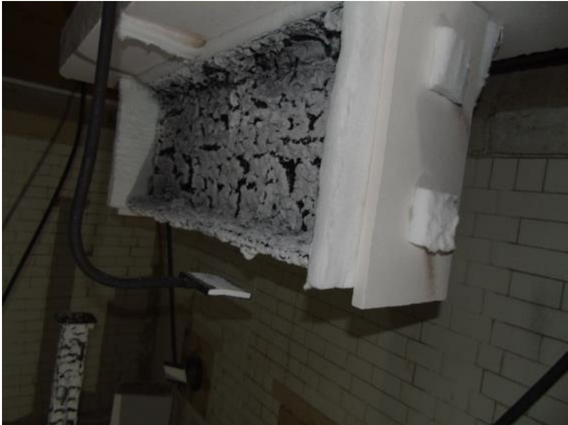
Photo D.13 Test 2: Reference beam with maximum protection thickness after the test
