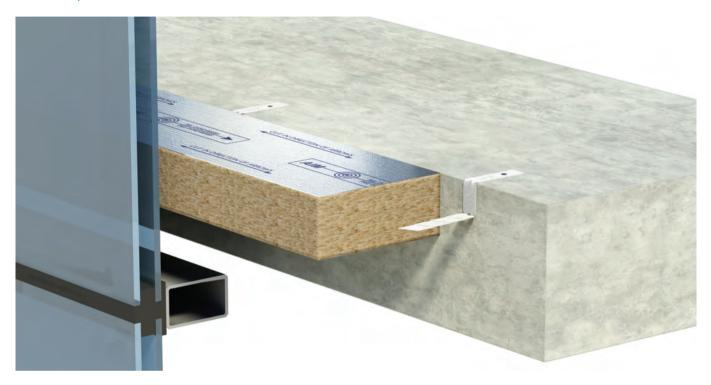
AIM Wall Cavity Barrier is made from foil faced high density Rockwool stone wool and is suitable for use in all cavity walls, as well as for fire stopping between a curtain wall system and a concrete floor slab. The barrier prevents the passage of flame and smoke within the cavity it fills for a range of fire rating periods as detailed in the table below.
